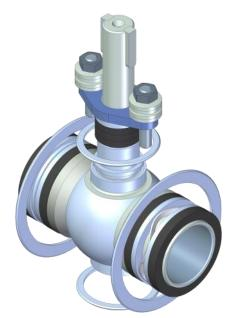
All metal seats are wide faced large contact area designs. Although this results in more torque requirement, the design is resilient to leakage and has proven to perform reliably in harsh process conditions. The seat face may be either hard chrome plated, cobalt alloy overlay, tungsten carbide or chrome carbide.
